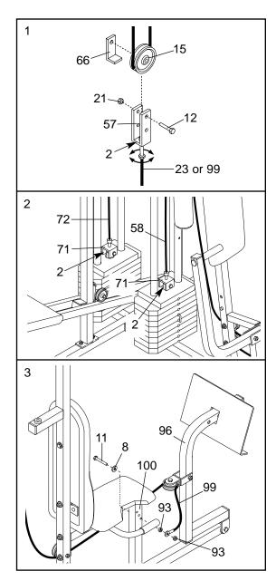
If a cable tends to slip off the pulleys often, it may have become twisted. Remove the cable and re-install it.
